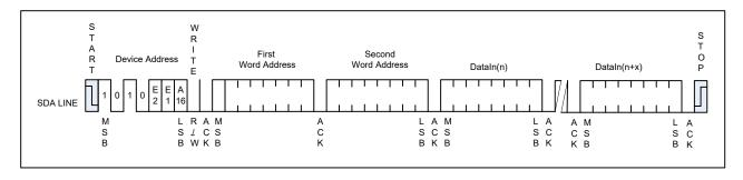
The lower eight bits of the data word address are internally incremented following the receipt of each data word. The higher data word address bits are not incremented, retaining the memory page row location. When the word address, internally generated, reaches the page boundary, the following byte is placed at the beginning of the same page. If more than 256 data words are transmitted to the P24CM01H, the data word
