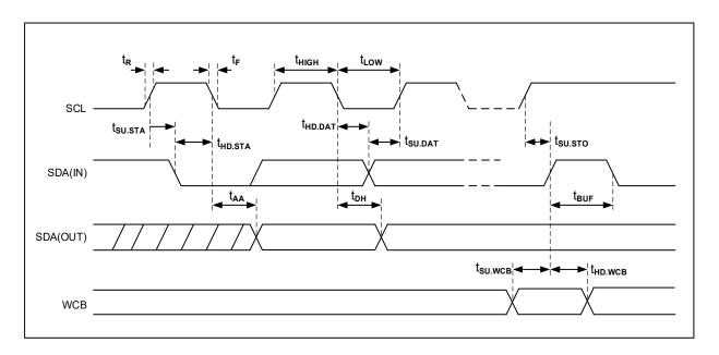
**Figure 3-2 Write Cycle Timing**
